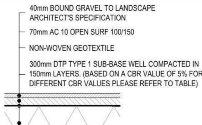
TYPE 5 - RESIN BOUND GRAVEL (FLEXIBLE) (ST ALBAN'S PLACE) SCALE 1:20
